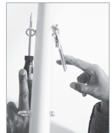
Figure 9: Use two fingers to tighten bolts
