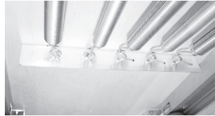
Figure 3: Springs hooked downward
