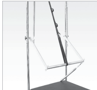
Figure 7: Safety strap holding the push-through bar at 4 o'clock. The strap is secured to the PTB and canopy frame, not the eyebolts.
